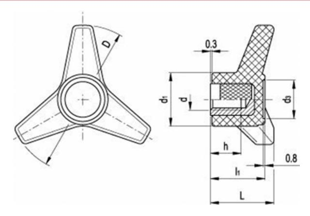
$\begin{array}{lll} D & = 80 \\ d1 & = 32 \\ d3 & = 21 \\ dh & = M10 \\ h & = 17 \\ I1 & = 30 \\ L & = 35 \\ Weight in (g) = 61 \end{array}$
